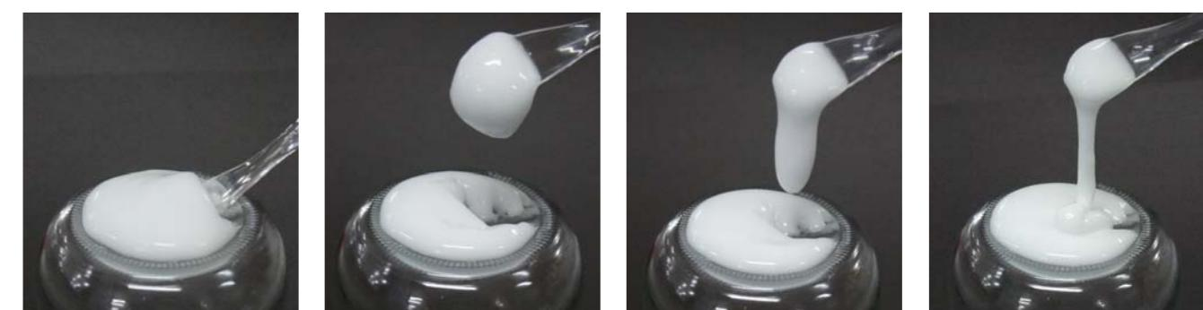
Mixed with 20 parts of oil and 80 parts of GT-700 2%aq. , and the mixture was stirred for 5 minutes at 10000rpm homomixer at 25°C.
